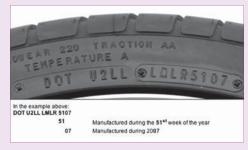
For example, LMLR5107 means the tire was manufactured in the 51st week of the year 2007.
